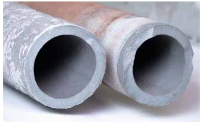
SiC rollers after 12 months - Superficial contamination with no penetration into the body
