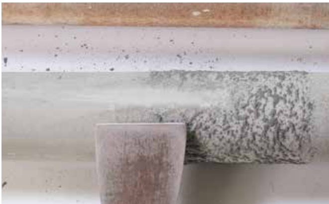
SiC rollers after 12 months - Superficial contamination with no penetration into the body
